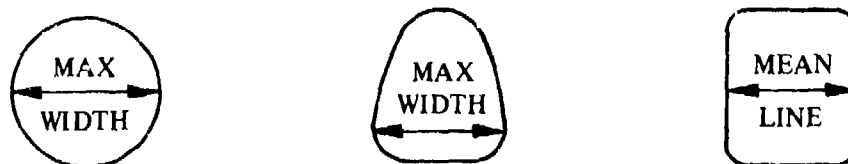
SEVERAL FUSELAGE CROSS-SECTIONS SHOWING CAMBER LINE VERTICAL LOCATION
